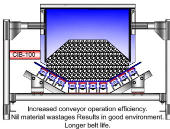
Sturdy support cradle. Compatible to all trough angles. Cradles offered for Medium and Heavy duty Applications. Impact bars of 60 mm and 75 mm thickness offered for application suitability.
