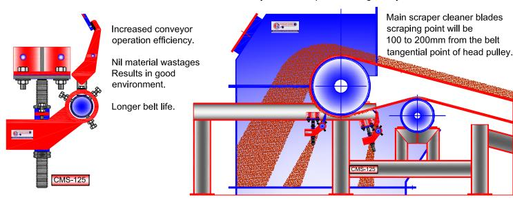
Cleaner blades like High Grade Tool Steel, Tungston Carbide Tip blades, Stainless Steel blades depends on material characteristics. Suitable for High temperature Applications. maintaining effective constant pressure for better cleaning. Recommended for moisturized and sticky materials. Suitable for high capacity, high speed belts with larger head pulleys. Cuts sticky material to material adhesion.
