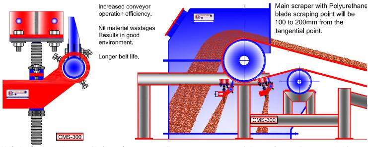
PU blades flex in the direction of belt travel maintaining effective constant pressure for better cleaning. Recommended for moisturized and sticky materials. Suitable for high capacity, high speed belts with larger head pulleys. Cuts sticky material to material adhesion.
