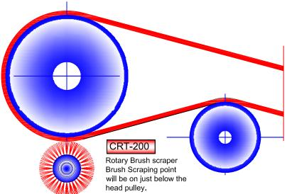
Nylon Bristle of Rotary Brush rotates in the opposite direction of belt travel with speed of 2 to 2.5 times of the belt speed for maintaining effective cleaning. Recommended for dry and calcined materials up to 80° C and suitable for moisturizes non sticky materials provided with external pre scraper model CPS-125. Suitable for high capacity, high speed belts with larger
